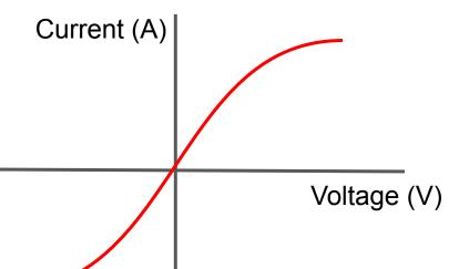
When current flows, the filament produces heat. This increases the resistance of the filament (R=V/I).
