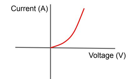
Current through a diode flows in one direction only, as it has a very high resistance in the opposite direction.
